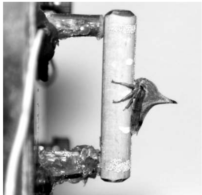
Fig. 1 Bending wave simulator consisting of a section of wooden dowel (length 3.0 cm) driven by two piezoelectric actuators. A female Umbonia crassicornis is at the center of the dowel. The laser was positioned approximately 20 cm opposite the center of the dowel, and thus measured motion in the plane of the long axis of the actuators and the dorso-ventral axis of the insect
